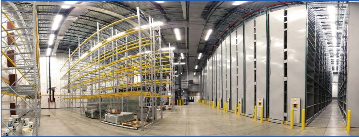
← Panoramic view of Bulk Storage pallet racks and 35' tall SpaceSaver Xtend moveable aisle shelves.
